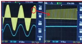
Fig. 15 chopper circuit output @ 20 kHz PWM frequency
